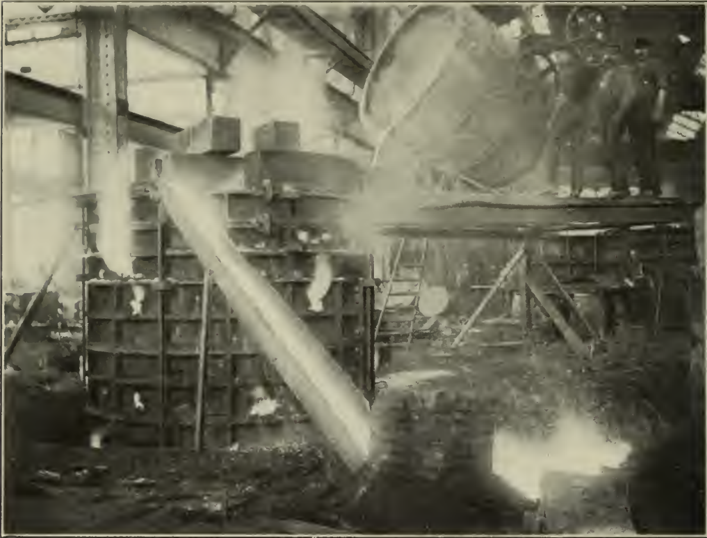
POURING A CROSS-HEAD GUIDE, WESTINGHOUSE MACHINE CO.
